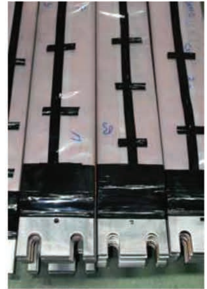
The copper or aluminium conductor is insulated with 4 layers of 125-micron polyester film.
